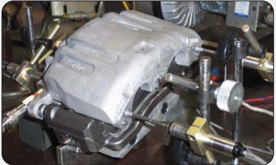
Above: All FRBC calipers hit the designed stiffness prediction with 25% increase over the baseline Bottom left: Good fatigue response on all tested calipers – FRBC averaged over 150,000 cycles at 16MPa loads
