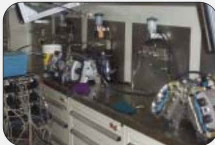
Above: All FRBC calipers hit the designed stiffness prediction with 25% increase over the baseline Bottom left: Good fatigue response on all tested calipers – FRBC averaged over 150,000 cycles at 16MPa loads
