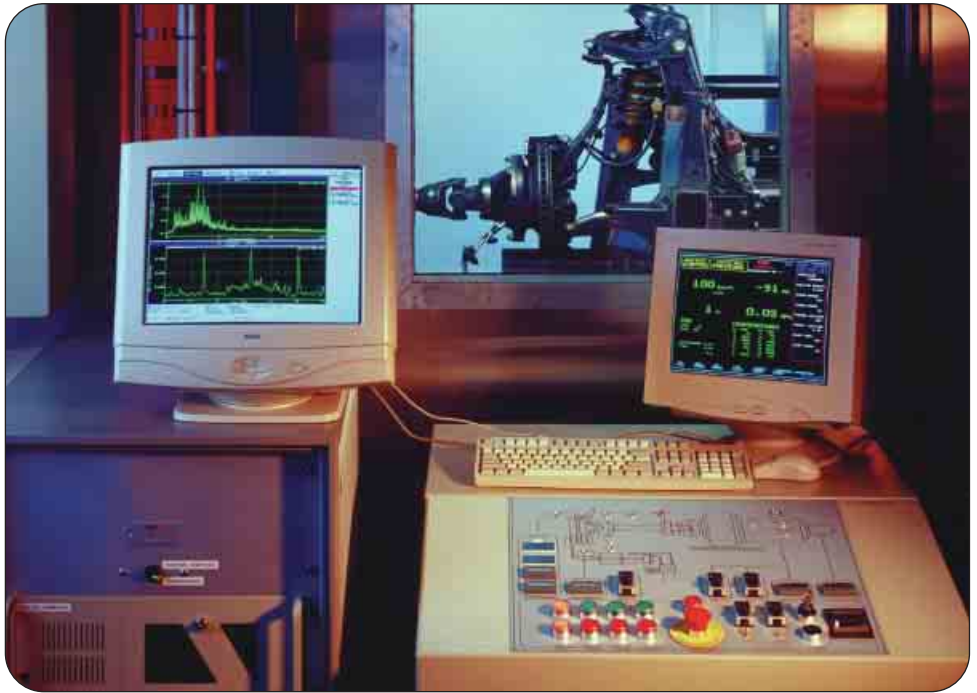
A PBR noise dynamometer conducts noise testing.
