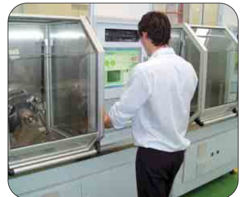
Torque durability tests provide essential caliper information.
